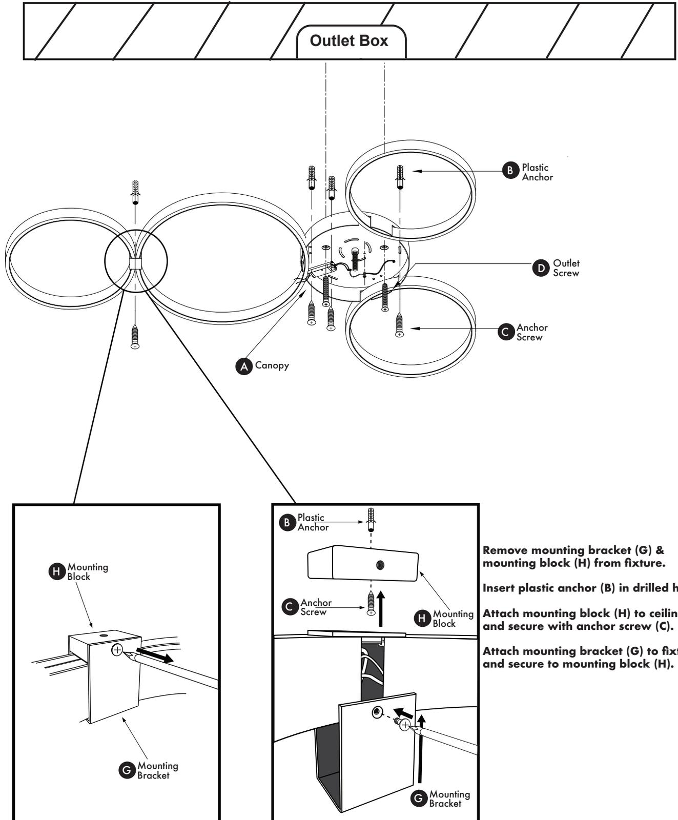
Remove mounting bracket (G) & mounting block (H) from fixture.
