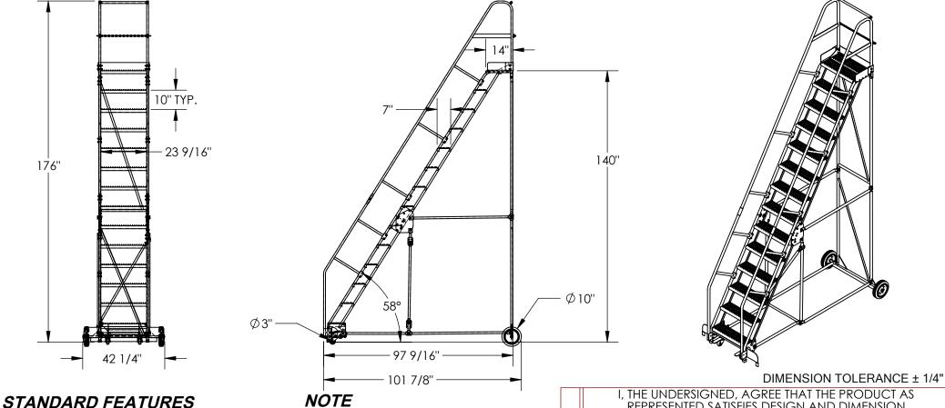
MODEL NUMBER IS LAD-14-14-G OVERALL WIDTH IS 42 1/4" USABLE WIDTH IS 23 9/16" **OVERALL LENGTH IS 101 7/8" USABLE LENGTH IS 97 9/16" OVERALL HEIGHT IS 176"** TOP STEP HEIGHT IS 140" STEP TYPE IS GRIP STRUT CLIMB ANGLE IS 58° STEP DEPTH IS 7" TOP STEP DEPTH IS 14" MAX CAPACITY IS 350 LBS
