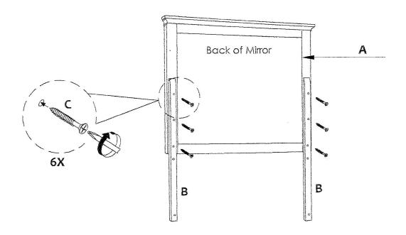
Align the Marking Line with the Mirror Back Support (B) at back of Dresser (as shown) and secure it with CSK Screw (C) using Phillip Head Screwdriver ( Not included)
