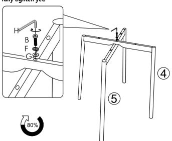
**Loosely** attach the bolts (D) one by one and **keep them loose. Do not fully tighten.** After **loosely** attach the first bolt, move on to the diagonal bolt. After all 4 bolts are attached, use allen wrench (H) to tighten.
