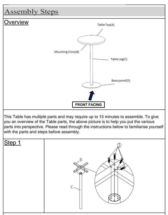
Open the carton and place all the parts onto a clean, non-marring surface. Attach the Mounting Cross(B) to Table Leg(C)using Hardware(1) with Allen Key(2) as shown in Picture .
