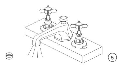
After installing faucet, open the hot and cold supplies to check for leaks. Turn on faucet handle for one minute to flush debris from faucet. Turn off the handle.
