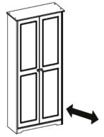
To move doors in or out: loosen screws shown and move doors to suit. Re-tighten screws.
