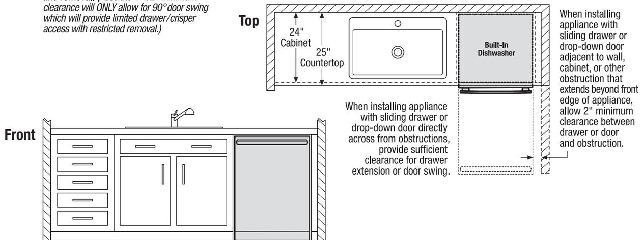
When installing appliance with sliding drawer or drop-down door adjacent to wall, cabinet, or other obstruction that extends beyond front edge of appliance, allow 2" minimum clearance between drawer or door and obstruction.
