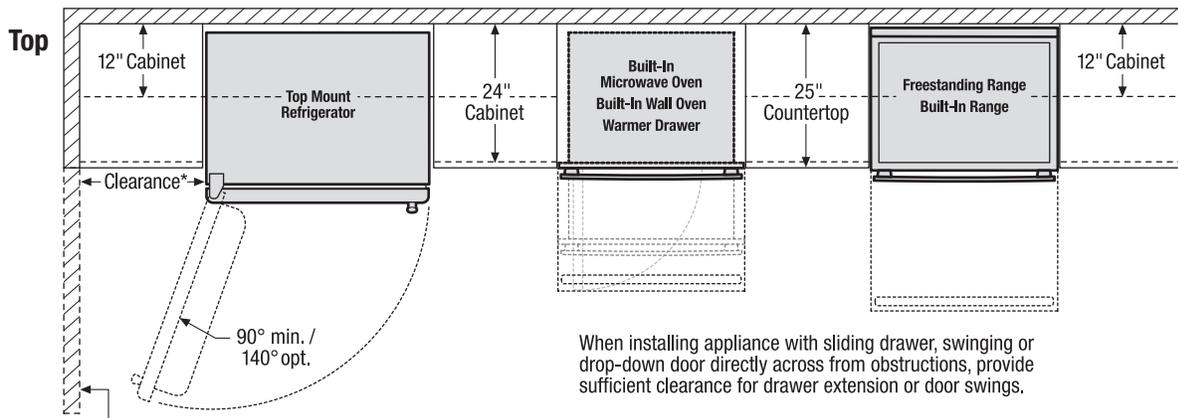
\*When installing top mount refrigerator adjacent to wall, cabinet or other appliance that extends beyond front edge of unit, 20" minimum clearance recommended to allow for optimum 140° door swing, providing complete crisper access and removal. (Absolute 3" minimum clearance will ONLY allow for 90° door swing which will provide limited crisper access with restricted removal.)
