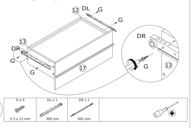
Fix runner(DL) and (DR) to plate 12 and 13 using screw(G) as shown.
