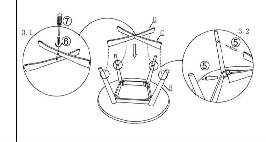
First, fix the connecting rods (C) and (D) with a screwdriver (7) and Rapid tooth (6), as shown in Figure (3.1). The wooden tenon (5) is inserted into the connecting rod (C) (D) and the table leg (B), as shown in Figure (3.2).
