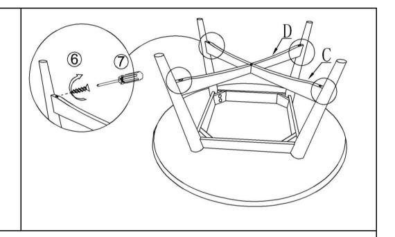
Secure connecting rod (C) (D) and table leg (B) with Screwdriver(7) and Rapid tooth (6), as shown in the figure. Finally, tighten all the screws.
