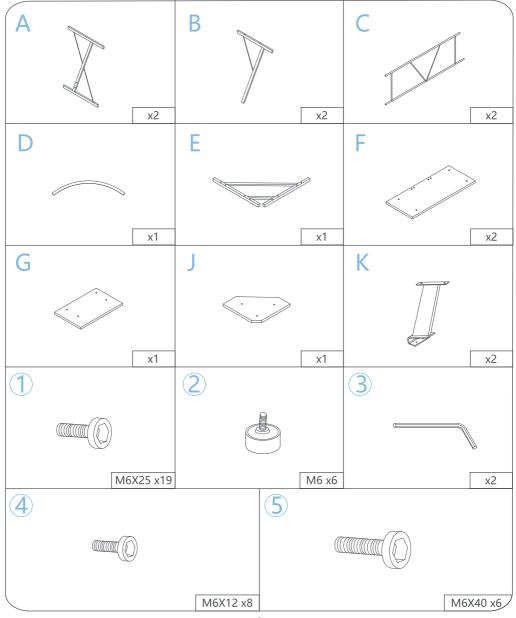
Install the A and E by tightening all screws ① to 100% tighteness.
