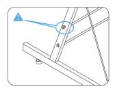
6. Check the firmness of the screws and other metal parts regularly.
