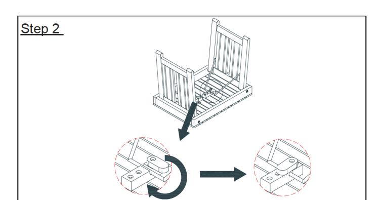
Rotate the Wooden Lock 90 degrees to lock Leg Supports into position.
