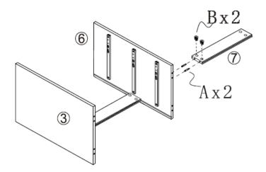
**Step 6:** Connect Panel 4 to panel 7 using hardware A and B.
