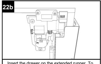
Insert the drawer on the extended runner. To secure the drawer clips with the runner, push the drawer in. Upon successful locking, a click can be heard.
