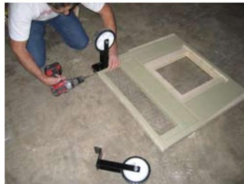
Fasten wheels on the bottom as shown with 2 1/2" deck screws.
