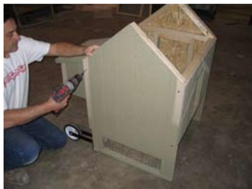
Attach the wall with the wheels and secure with 1 1/4" screws as shown.
