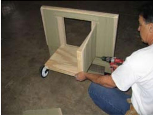
Install the nest side panel as shown and secure with 1 1/4" screws.
