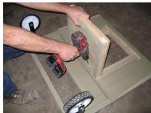
Secure with 2 1/2" screws as shown.
