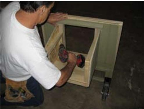
Make sure the opening is flush on the inside and secure with 2 1/2" screws.
