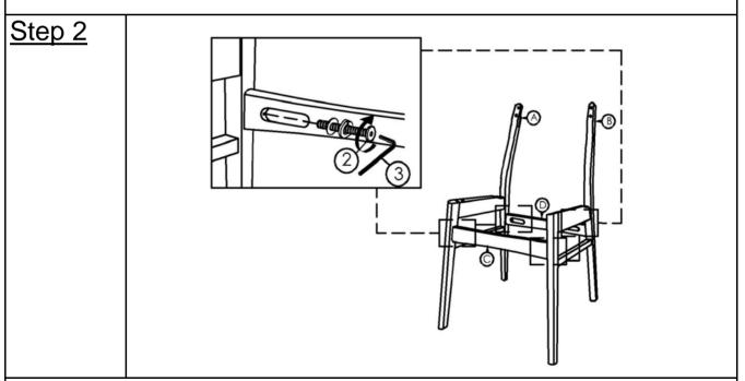
Then, fix the Front Scretcher (C) and Back Sctretcher (D) with JCBC Bolt ② + Spring Washer + Flat Washer using Allen Key ③.
