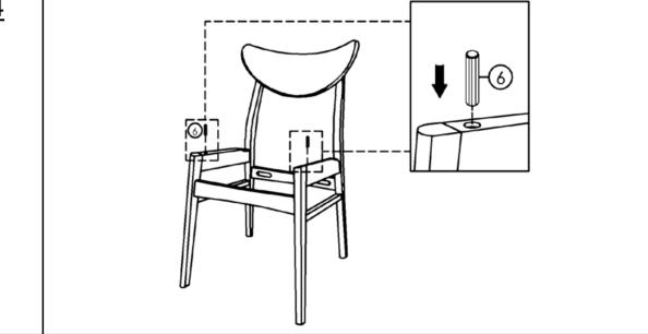
Place Wood Dowel 6 on the Side Frame as shown above.
