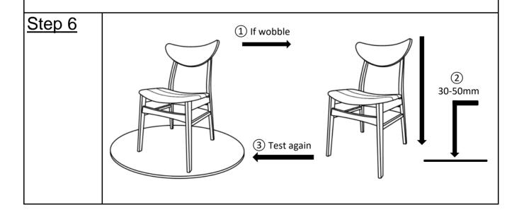
Place the dining chair on a Level Surface to check if it wobbles. loosen the bolts. lift the dining chair some 30mm to 50mm high from the ground, keep your feet and toes well away from the drop zone, and drop the dining chair freely and vertically with the four legs, hitting the ground at the same time. This Drop Test will help to ensure that all the bolts and gaps to all reach full alignment.
