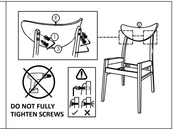
Place the Top Rest (E) on the back frame as shown above.
