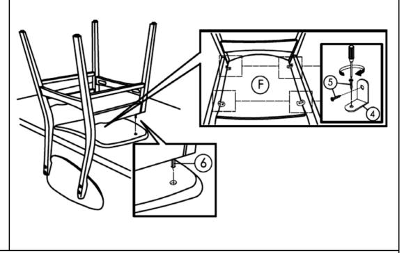
Place **the Cushion Seat (F)** on the table, then put the assembled chair parts in Step4 to fix the Cushion Seat (F) as shown.
