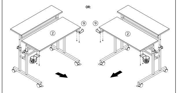
Finally, set the tabletops to the height of your preference, and proceed to tighten all the screw knobs (G).
