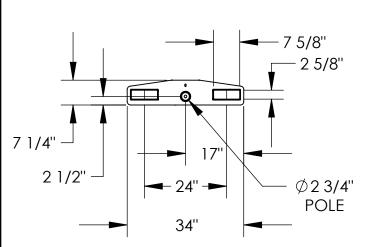
HORIZONTAL CENTER OF GRAVITY: 62 7/8" VERTICAL CENTER OF GRAVITY: 2 15/16" LOST LOAD: 437 LBS. (APPROX.)
