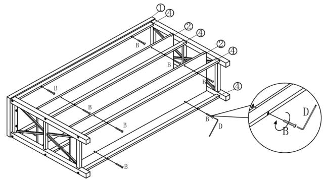
Important note: If you find the holes do not align together, you can loosen all the screws (A & B & C), and then you can adjust the holes slightly. After all the holes were aligned together, you can fully tighten all the screws.
