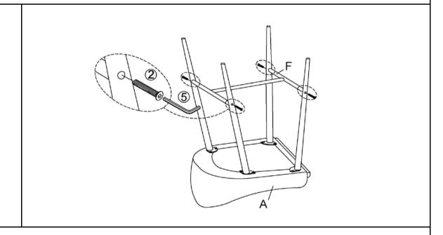
Attach Connecting Tube(F) to Leg 1(B), Leg 2(C), Leg 3(D) and Leg 4(E) using Bolts(②) with Allen Key(⑤) as shown above.
