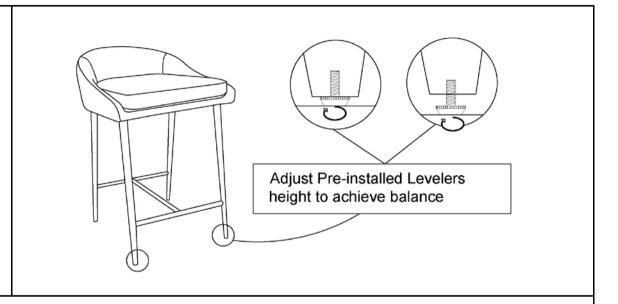
Adjust the Pre-installed Levelers on the bottom of Leg 1(B), and Leg 2(C) until the Stool is level with the ground.
