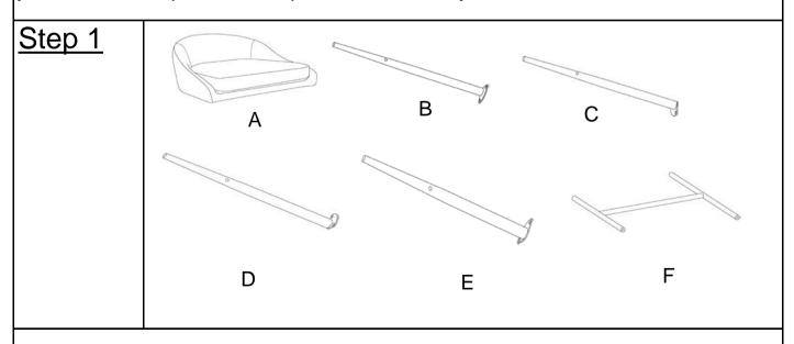
Place the Cushion(A), Leg 1(B), Leg 2(C), Leg 3(D), Leg 4(E) and Connecting Tube(F) onto a clean, non-marring surface.
