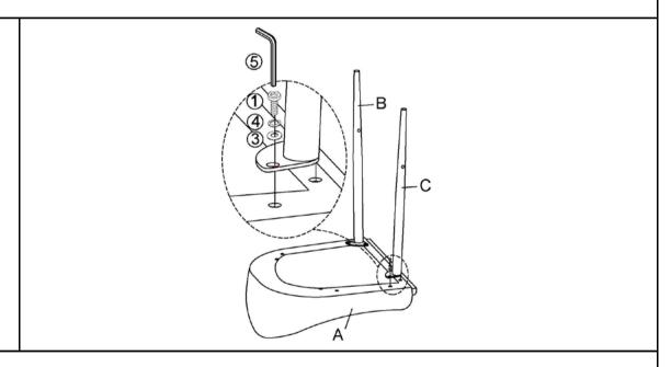
Attach Leg 2(C) to Cushion(A) using Bolts(1), Spring Washers(4), and Washers(3) with Allen Key(5) as shown above.
