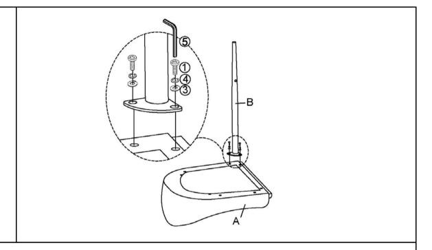
Align Leg 1(B) to Cushion(A) as shown above. Attach Leg 1(B) to Cushion(A) using Bolts(1), Spring Washers(4), and Washers(3) with Allen Key(5) as shown above.
