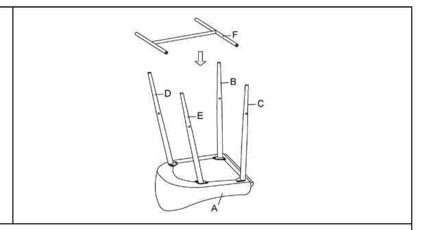
Align Connecting Tube(F) to Leg 1(B), Leg 2(C), Leg 3(D) and Leg 4(E).
