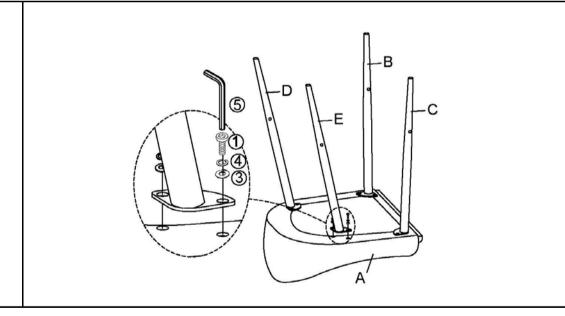
Attach Leg 4(E) to Cushion(A) using Bolts(1), Spring Washers(4), and Washers(3) with Allen Key(5) as shown above.
