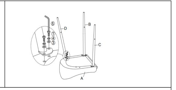
Attach Leg 3(D) to Cushion(A) using Bolts(1), Spring Washers(4), and Washers(3) with Allen Key(5) as shown above.
