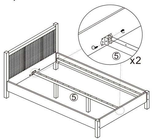
STEP 3 Attach the bed slats(7) with bed frame by hardware E(the connect hole were pre-drilled)
