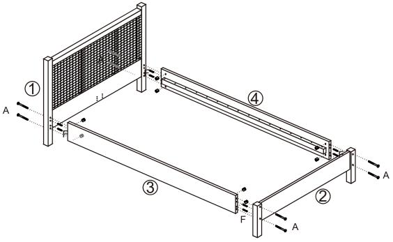
STEP 2 Attach hardware B by hardware C on headboard(1) and footboard(2).
