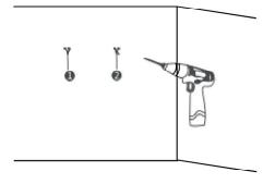
Punch 2 holes in the wall with an electriv drill at the proper height. The drilling location depends on whether you want to hang it horizontally or vertically.
