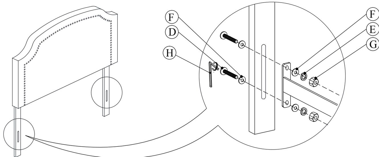
NOTE: AFTER A FEW DAYS OF ASSEMBLY, IT WILL HAVE ACCLIMATIZED TO THE ENVIRONMENT. PLEASE TIGHTEN ALL HARDWARE. CHECK TIGHTNESS OF ALL SCREWS EVERY 6-8 WEEKS.
