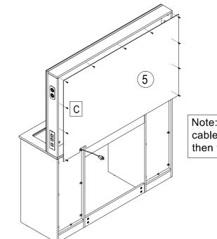
Note: Firstly drag the power cable out from the gap and then fix the mirror backboard.
