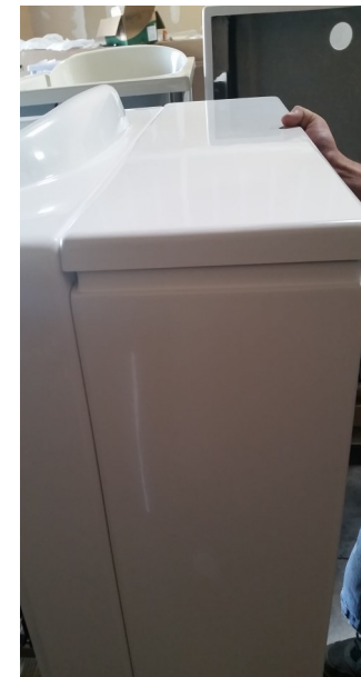
Place Top Piece over the Groove
