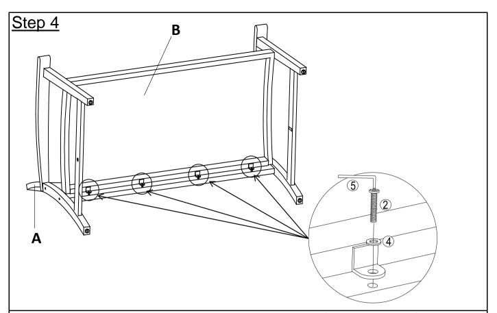
Secure Seat Panel (B) to Back Panel (A) using Bolt (2) & Washer (4) with Allen key (5)
