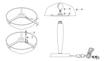
1. Adjust the two screws<sup>3</sup> on the three-pronged bracket<sup>1</sup> to loosen, fix the three-pronged bracket<sup>1</sup> on the glass lamp shade, and then use a screwdriver<sup>2</sup> to tighten the screws<sup>3</sup>.
