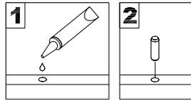
The dowels are necessary to attach assembly parts together in the following steps. Place a small amount of glue on the end of the dowel before attaching parts together. Please remember wipe away the excess glue immediately.
