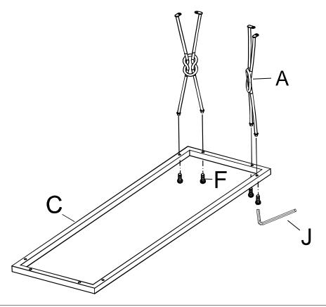
Attach Side Panel (A) and Middle Side Panel (B) to Bottom Frame (C) by Bolt (F) and Allen Wrench (J) as shown.
