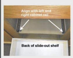
For both rails, slide the INNER ball bearing carriage all the way forward to the stop, then insert the slide-out shelf or organizer into the cabinet rails as shown and test the in and out glide motion to be sure it is smooth, not too tight and not too loose.
