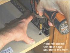
Position the rails between the template to be parallel and square to the front of the shelf/cabinet, making certain both inner rail extenders clear the opening by sliding them out and back in. Using the #6 x 5/8" pan head screws provided drive a screw thru the small **round** hole in both the front and rear L-brackets of the right rail. Do not use the oval holes.
