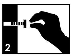
Position each part correctly and insert all screws into their respective holes. Then, hand-tight and leave room for later adjustment. Do not use tool.
