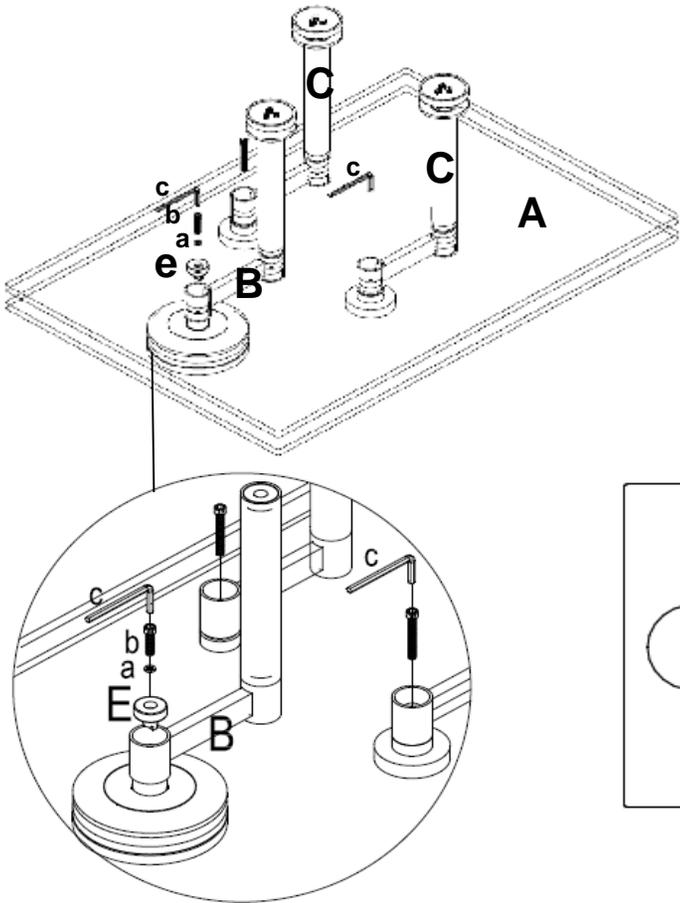
**Noted:**The direction of the footpillar should be paralld.
