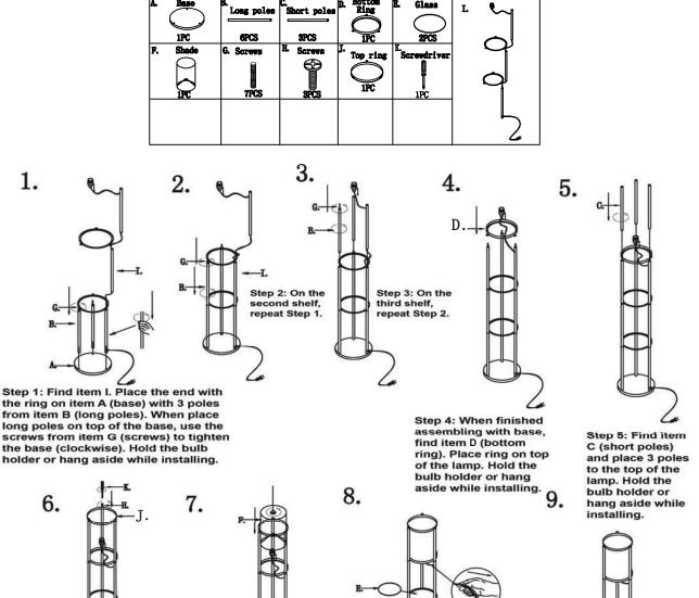
Step 6: Find item J (top ring) and place at the top of the lamp. Use screws from item H to tighten top ring. Hold the bulb holder or hang aside while installing.
