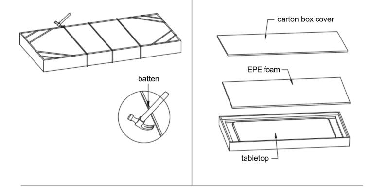
1. Use a hammer to carefully pry the battens apart.
