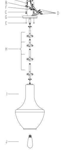
PLEASE USE ON/OFF TYPE"A" BULB MAX 60-WATT OR CFL BULB MAX13 -WATT OR LED BULB MAX9 -WATT THERE ARE LED 1PCS 4-WATT BULB IN THE BOX
