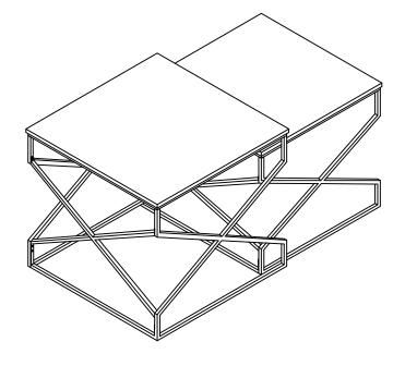
STEP 2. Put the Marble top (A) on the top of Metal base (B) and make sure it is in the correct location as diagram shown.
