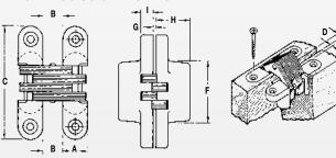
All SOSS Hercules Hinges are shipped with the proper size wood and machine screws unless ordered without. Do not exceed "E" dimension.
