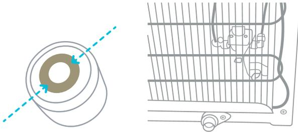
7. Locate the second Small PE Tubing. Connect one end of the Small PE Tubing to the right side inlet of the right Filter Adapter. Connect the other end of that Small PE Tubing to the water inlet (#18).
