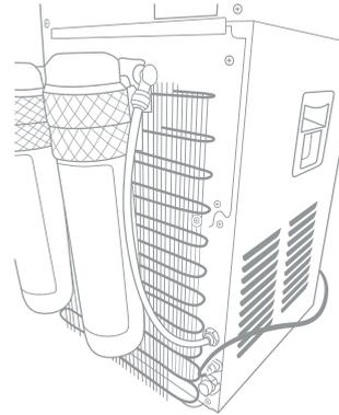
8. Locate the valve on the Valve and Tube Assembly. Turn this valve to the on position (parallel to the PE Tubing) to allow water to flow through.
