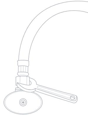
3. Connect the Metal Adapter with valve between the cold water supply line and cold water valve.
