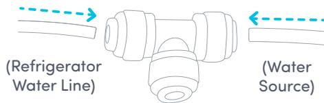
4. Insert one end of the PE Tubing that is supplied with the water cooler into the third opening of the Three Way Plastic Adapter.
