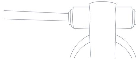
3. Hold the filter with the Filter Flushing Adapter in place over a sink. Turn the Valve of the Metal Adapter at the water source to the on position (the on position is parallel to the PE Tubing) and allow the water to flow through the Adapter and the filter for approximately 2 minutes to flush the new filter.
