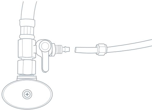
5. Screw the nut tightly into place to keep the PE Tubing securely connected to the Metal Adapter with Valve. Make sure the valve is in the off position (perpendicular to the PE Tubing).
