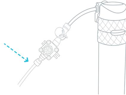
5. Using the Small PE Tubing, connect the right side inlet of the first Filter Adapter to the left side inlet of the second Filter Adapter.
