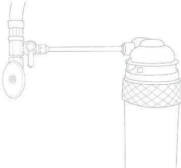
5. Remove the end of the PE Tubing from the Filter Flushing Adapter by pressing in on the push connect ring and pulling out the PE Tubing.
