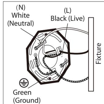
4. Connect (push) electrical wires from fixture into correct inserts.
