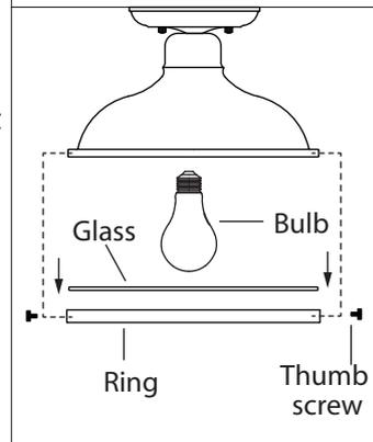
6. Install proper bulb type and wattage (not included).
