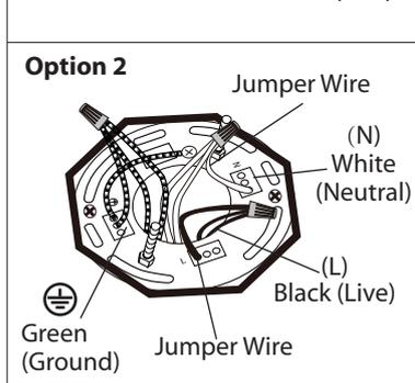
3. **Option 2:** For multiple green (ground), black (live) and white (neutral) wires joined in the electrical box (house wiring), attach a single "green", "black" and "white" jumper wire before connecting. Strip 7mm from the 6" jumper wires (AWG 12-24) supplied. Then connect (push) wires into the correct inserts.
