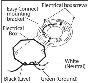
2. Attach easy connect mounting bracket to electrical box with electrical box screws (not included).
