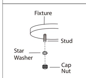
5. Tuck electrical wires into electrical box and position fixture over studs on mounting bracket assembly. Secure fixture in place with star washers and cap nuts.
