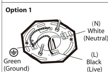
3. **Option 1:** Connect (push) electrical wires from electric box (house wiring) into correct inserts.
