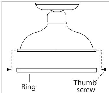
1. Unscrew the 3 thumb screws to remove the ring.
