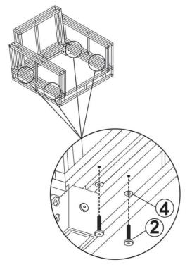
Do not fully tighten hardware until all components in this step have been connected.
