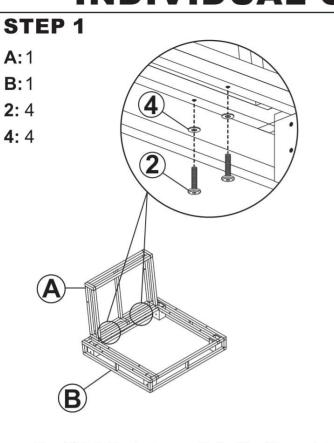
Do not fully tighten hardware until after Step 3 is complete.
