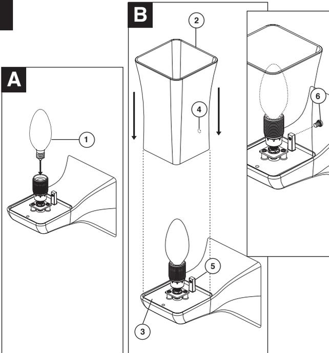
**A.** Install candelabra style bulb (1) with E12 (small) base, 60 watt maximum.
