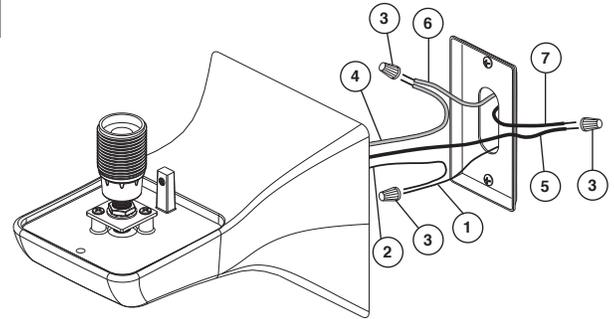
Feed the wires through the center hole of the plate. Connect house ground wire (1) to the fixture ground wire (2) using the supplied wire nut (3), or if there is no house ground wire attach fixture ground wire to mounting plate with ground screw provided. Connect the white wire (4) of the fixture to the house white wire (6) with a wire nut (3) and the black wire (5) of the fixture to the house hot black wire (7) with a wire nut (3).
