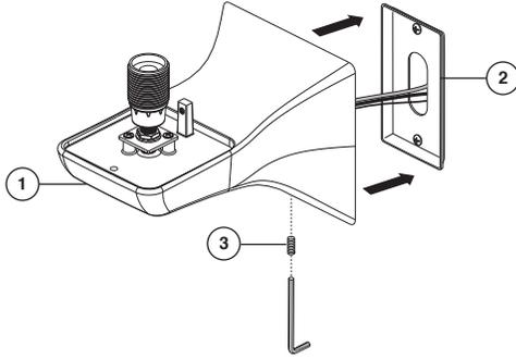
Place the fixture (1) over the plate (2) until it is flush against the wall. Take care wires are not pinched during this process. Secure the fixture by tightening the set screw (3) on the bottom side of fixture.
