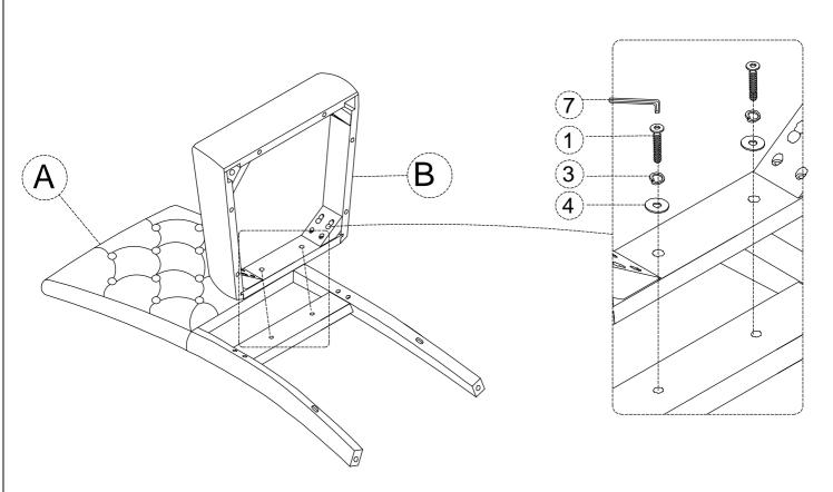
Bolts | Spring Washer | 1/4"x 13mm x 1.5mm | Flat Washer | 1/4"x 16mm x 1.5mm | Allen Key | 4mm x 60mm | 4mm
