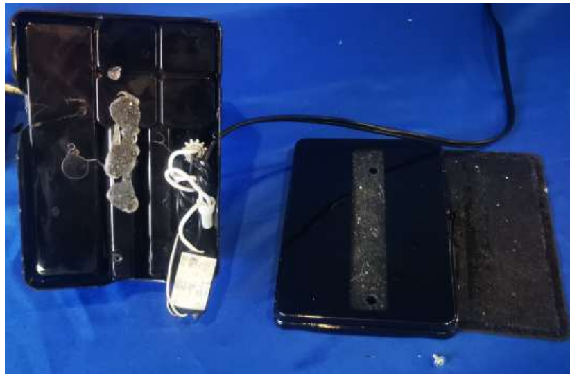
Photo 8 - Bottom view of model AF49481BK (Remark: Connector will fully cover by heat-shrinkable tubing)
