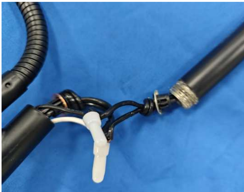
Photo 18 – Internal view of model CX00002BK, also represents model F9007. (Remark: Connector will fully cover by heat-shrinkable tubing)
