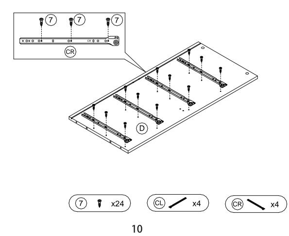
Attention: The hole positions are different when installing the slide on the front and back of the board C.
