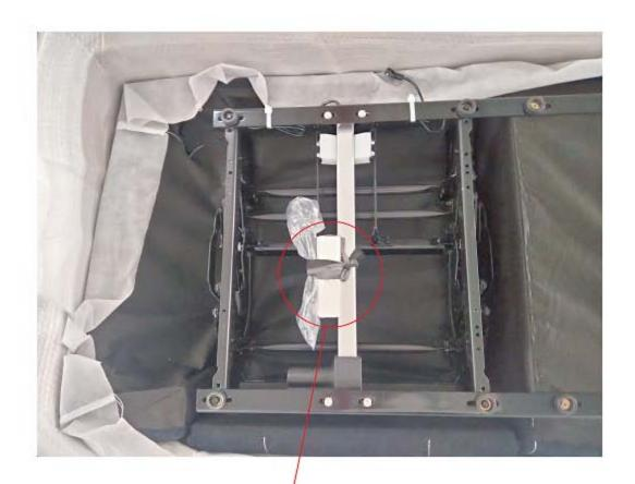
Loose the strap, connect the plug to the socket.
