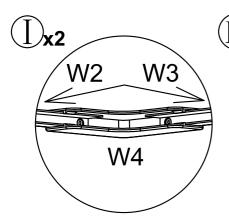
Insert the other end of W2 and W3 into corner guard W4.
