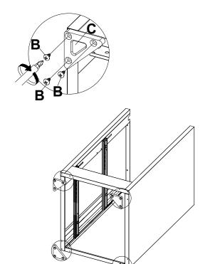
Put twelve screws to hold part C into place
