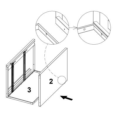
Put three screws to hold part 2 and 3 into place
