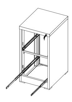
1.Pill out the small rails in the slide rails on the side walls completely. with two people lifing each side of the drawer, align the four divots on the bottom with the two rail clips on the rails on each side and insert them into the rail clips 2.After placing the drawer on the rail ,press the drawer base down hard enough, paying attention to check the position of the four clips inside until you hear a click four times, which means the drawer is in place
