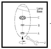
Parts A, B, C → are pre-installed under the tube
