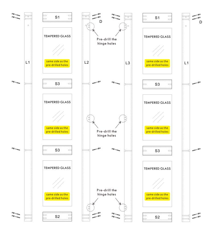
Install the left door with the back side as the reference.
