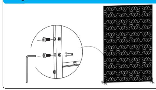
8.Use accessory M to fix base B and accessory E on the ground.
